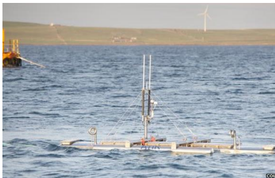
Figure 3. Installed and submerged tidal turbine
